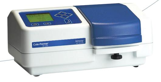
The SP-200 series spectrophotometers include model SP-200-VIS that covers the visible region of the spectrum, SP-250-VIS model with domed lid, and model SP-200-UV that uses a pulsed xenon lamp to extend the wavelength range into the UV region of the spectrum. All models have measurement modes for absorbance, percent transmittance and concentration. This makes the spectrophotometers ideal for basic photometric applications in schools and colleges, as well as in quality control laboratories.
